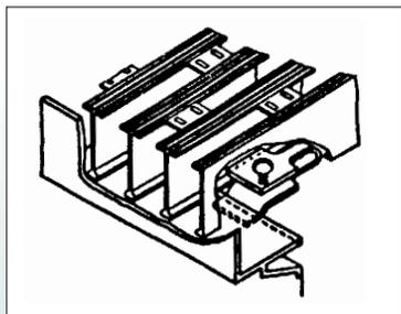
field. Frames can be provided in the mill finish condition or powder coated to protect surfaces which will come into contact with concrete.
